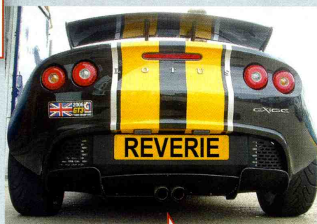
FIGURE 1 An exhaust system that exited above the diffuser allowed a clean exit for the airflow from the central diffuser section
